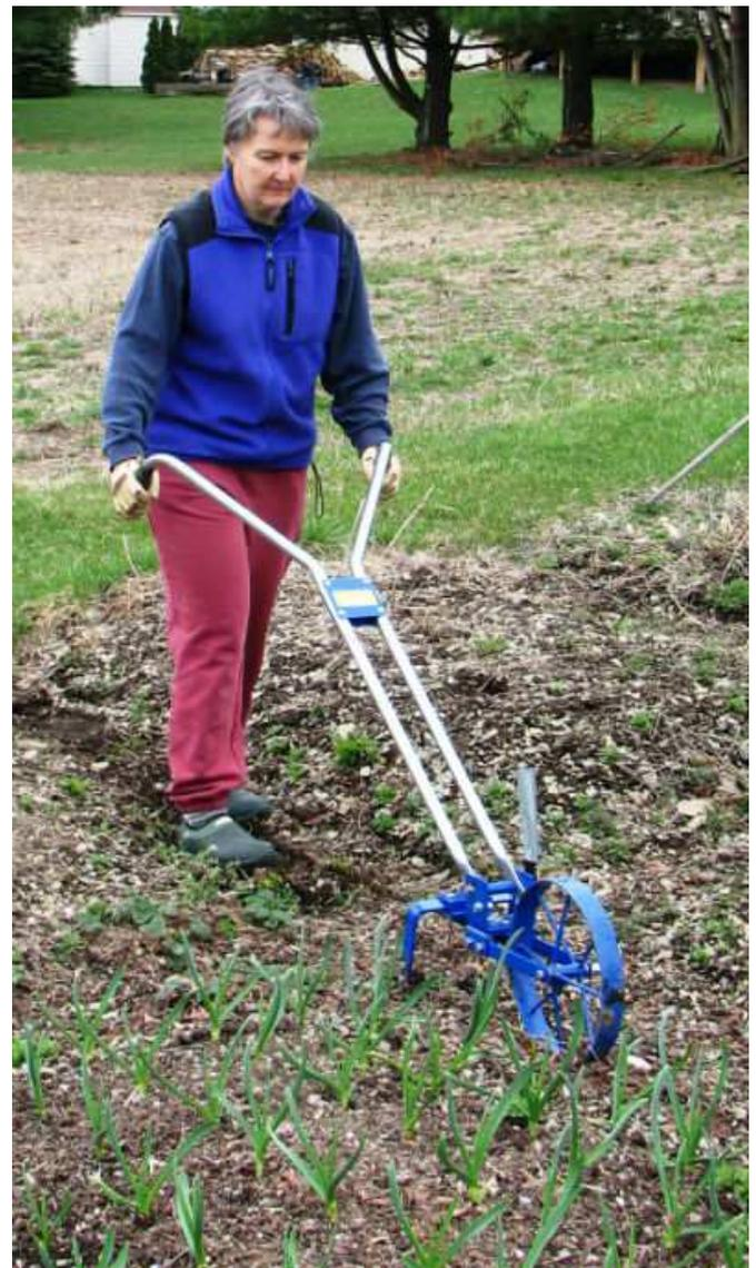
1 Green Heron Tools co-owner Ann Adams prepares a field for planting using a prototype of the company's new tiller. More than 3 years in development, the tiller utilizes a patent-pending technology that allows for battery-powered, vibration-free operation. Lighter and easier to maneuver than traditional rototillers, the tiller is undergoing rigorous testing and will likely
